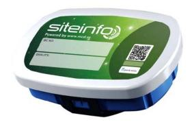
Together with our cloud service Sitelnfo, you can plan the perfect logistics and avoid empty IBC-containers. The sensor reads the data and saves the level every hour – the report is sent once per 24 hours. The frequency of reporting can be increased if necessary, but then at the expense of battery life.
